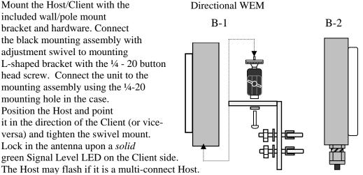
NOTE: The WEM antenna must be mounted as depicted above (Fig B-1 & B-2) to preserve its weatherproof capability. The RJ-45 port must be protected by the port plug and positioned underneath to prevent moisture pooling. Tighten weatherproof strain-relief so that it is snug, however, the cable should be able to move.
